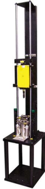
Figure 2.8: Instron 8200 Impact Tester (Dynatup, 2010)
