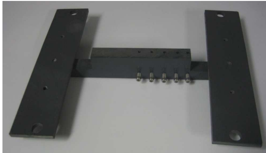
Figure 2.5: Thermocouple Holder (Bottom View) (Zantout, 2009)
